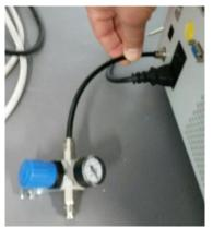
**Step 2**. Insert the other end of the short tube segment into the purge inlet located at the back of the thermal testing system.
