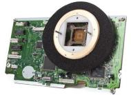
Elastomeric Frost preventing Armaflex Ring / Frost preventing Armaflex Ring placed between the Universal Adapter Plate and the board
