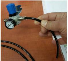
**Step 1**. Cut a small segment of around 20 cm in length from a black plastic tube with 0.6mm diameter. Insert one end of the short tube segment into a pipe connector of the pressure regulator.
