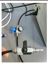
**Step 4**. Insert the other end of the long tube segment into the valve connector or regular connector of the dry air gas balloon. Follow manufacturer instructions for connecting to the dry air balloon.
