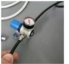
**Step 3**. Insert one end of the long segment of the black tube into the other pipe connector of the pressure regulator.
