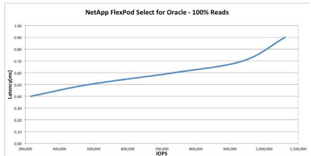
Figure 3) FlexPod Select for Oracle with eight RAC nodes showing 100% 8K random reads.
