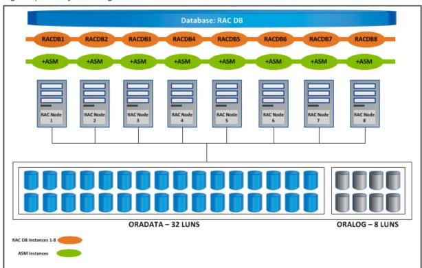
Figure 2) ASM layout for eight-node RAC.
