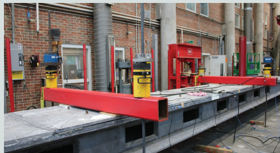
Figure 15. Test setup for the first flexure test of the floor slab.
