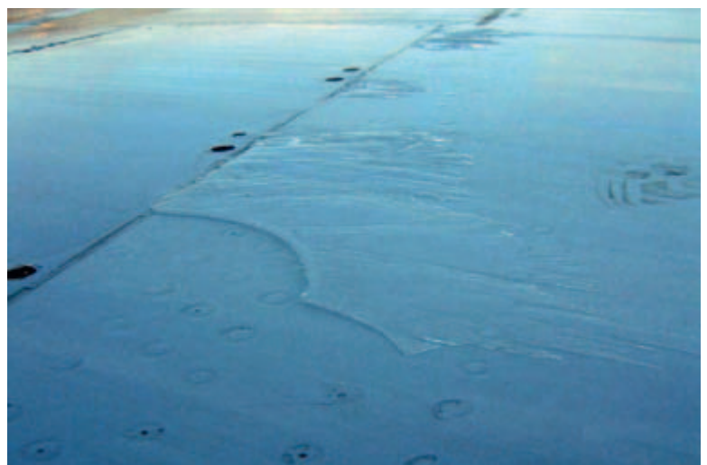
Figure 2 Clear-ice contamination on the wing
