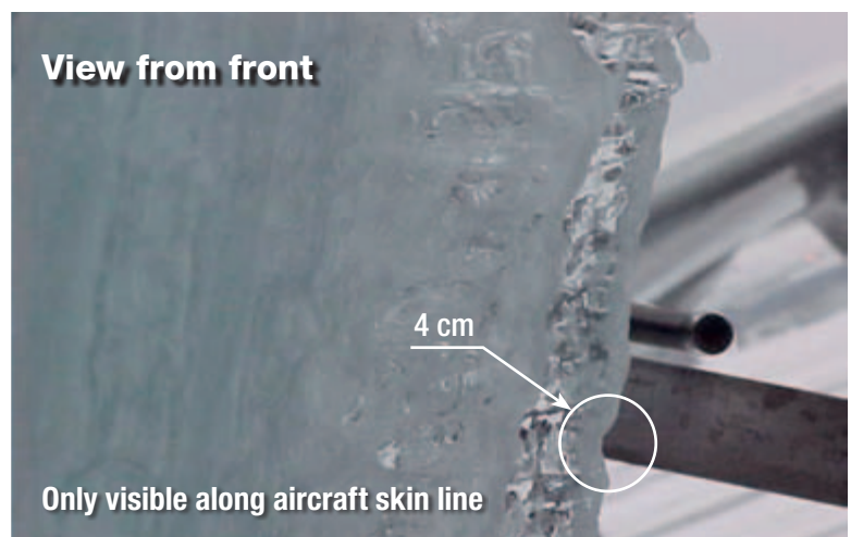
Figure 6 Ice bridge causing deflection of airflow away from pitot tube
