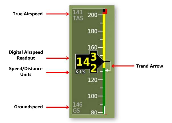
The instantaneous airspeed readout is contained in the black box with large, bold numbers. The digits appear to "roll by" smoothly as speed changes. The units of distance/speed are displayed below the digital readout. True airspeed (TAS) is displayed in the upper left corner, while GPS groundspeed is displayed in the lower left corner, as shown below.
