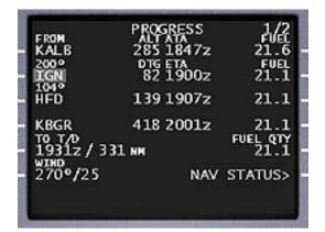
FROM / ALT/ATA/FUEL: The first line of the PROGRESS page display contains information related to the last flight plan fix that was over flown.
