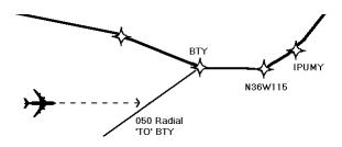
An Intercept Course entry is performed on the LEGS page. Enter the navigation fix that is desired into the scratch pad, the upselect the fix to the 1L LSK. This in effect tells the FMC/CDU that you are planning to cross that fix as the next point along your flight path.
