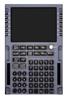
**FMC/CDU Display:** The MCDU display screen is comprised of 14 data lines capable of displaying 24 characters across in large or small font.
