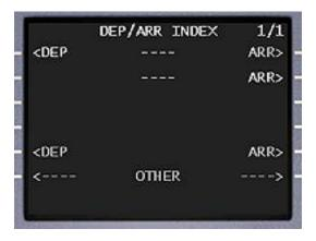
The DEP/ARR INDEX page allows the crew to select (using the appropriate LSKs) either the appropriate DEP procedure, or an ARR procedure for either of the two possible routes stored in the FMC
