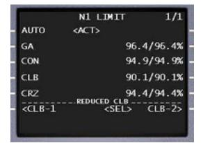
To select any of the various thrust limits available, simply press the associated LSK and the FMC/CDU will update the FMS to adjust the available thrust limit. Likewise, the CLB-1 and CLB-2 derated climb thrusts can be selected by pressing the associated LSKs near the bottom of the display.
