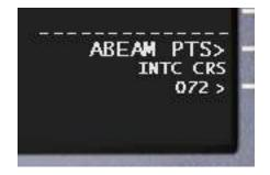
6R will show the current course to the desired waypoint. If a different intercept course is desired, it should be entered into the scratchpad, then up-selected to 6R by pressing the 6R key. This will instruct the FMS to intercept the desired course to the fix. The FMS will compute a great circle course between the current airplane location and the closest point of intercept to the desired course on the ND as a dashed white line.
