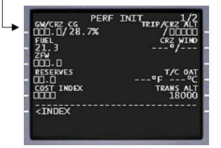
**LSK Prompts:** At any time a '<' or a '>' carat is used adjacent to a line select key, this indicates that an additional or related menu can be accessed by pressing the associated LSK. For example, the <INDEX prompt above indicates that pressing the 6L LSK will take you to the INDEX page.
