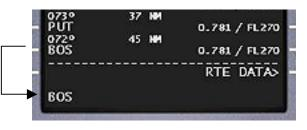
Then simply upselect the desired fix to the 1L LSK. This will cause the modified route to be displayed on the Navigation Display as a dashed white line, and will illuminate the EXEC key on the FMC/CDU to indicate that the route of flight change must be EXECUTED in order to take effect.
