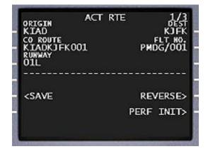
This will load the saved flight plan, and trigger the ACTIVATE> prompt so that crewmembers can confirm the route and EXEC it into active memory.
