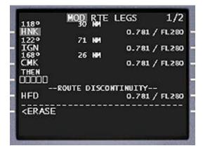
To confirm the continuation of the route, the waypoint identifier for the next fix in the desired route sequence should be downselected to the scratchpad by pressing the associated LSK. This fix identifier can then be up-selected to the line containing the disconnect prompt boxes. The FMC will then re-sort the flight plan to allow the updated routing.
