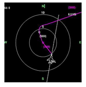
The fix that is currently the <CTR> cue in the FMC/CDU will be highlighted in white on the navigation display, and will be located at the center of the ND PLAN MODE display.
