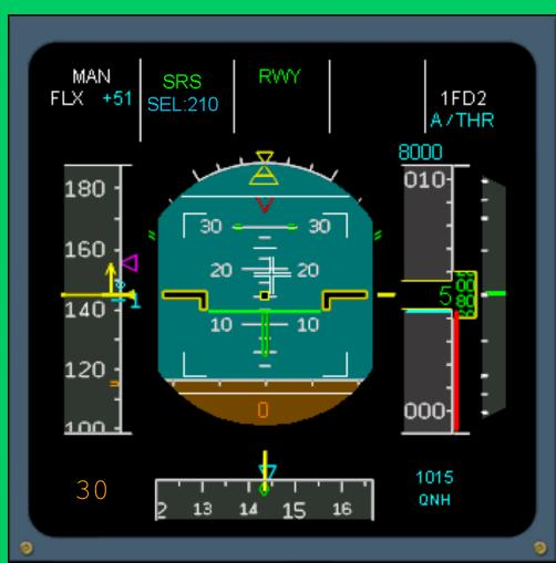
MAN SRS RWY CLB 210 NAV FLX 53 SRS MAN **CLB 210** FLX 53 In some A/C (AP-BGU & BGV) 180 when the thrust lever is set in FLEX/TOGA detent, Pre 160 Selected Climb Speed 210 Kts 20 · becomes armed (in Blue) & 140 CLB 210 is displayed on FMA. 10 This Pre Selected Climb 120 Speed 210 Kts was entered in the FMGC. SRS is engaged in 100vertical mode.
