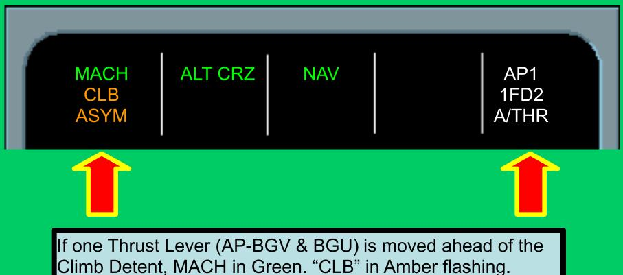
ASYM in Amber steady. Set the Thrust Lever in climb detent. A/THR remains Active (White).
