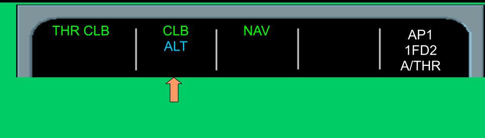
As the constraint is passed (we are in Managed Mode), Thrust goes to Climb Thrust (itself) and the aircraft resumes climb (itself). CLB becomes engaged mode and ALT armed, as FCU ALT is set at FL-290.
