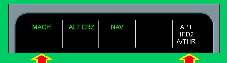
In a Normal Cruise, the FMA is as shown above. Both Thrust Levers are in Climb Detent. A/THR is Active (white).
