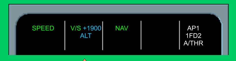
Pull the V/S knob on the FCU. We revert to SPEED and current V/S. NAV remains engaged.
