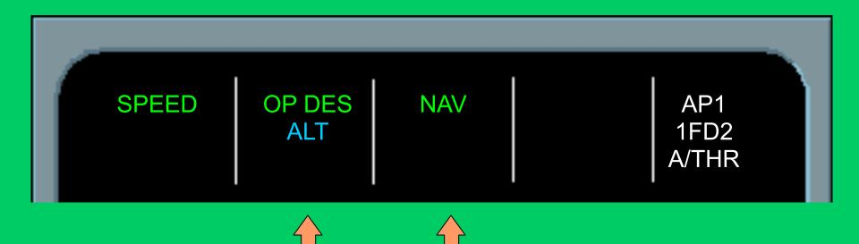
Pull the ALT knob to engage OP DES and capture the FCU selected altitude.
