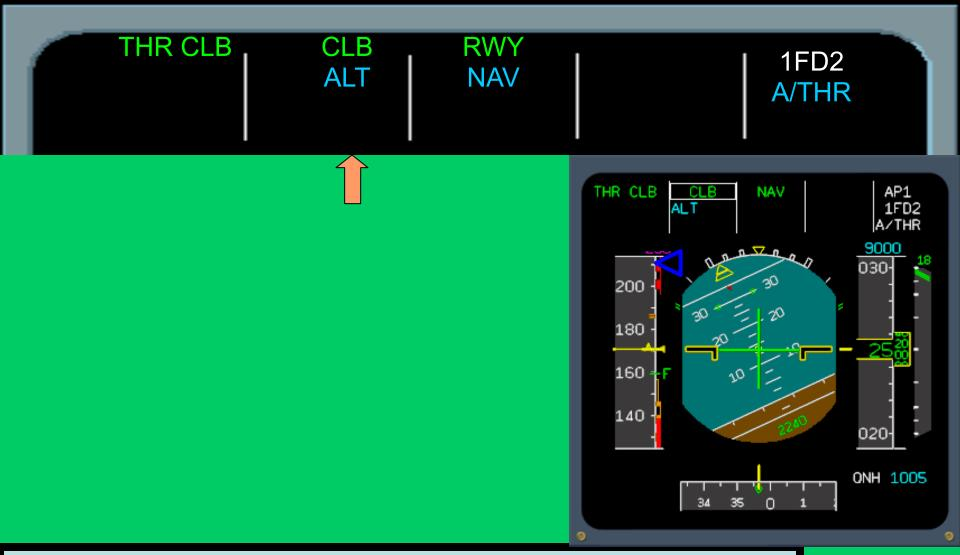
As SRS disengages (at Acceleration Altitude), on PFD speed target is 210 Kts shown as a selected blue ( ). CLB becomes the engaged mode and ALT becomes armed in Blue.
