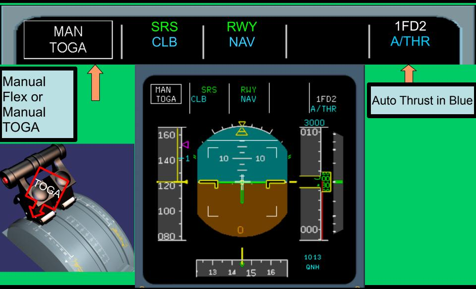
MAN FLEX or MAN TOGA engages when thrust lever is set in FLEX/TOGA detent. A/THR armed (In Blue)
