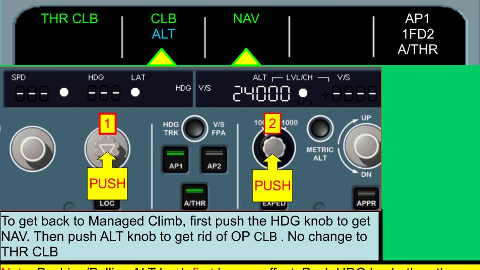
Note: Pushing/Pulling ALT knob <u>first</u> has no effect. Push HDG knob, then the ALT knob to get CLB/NAV
