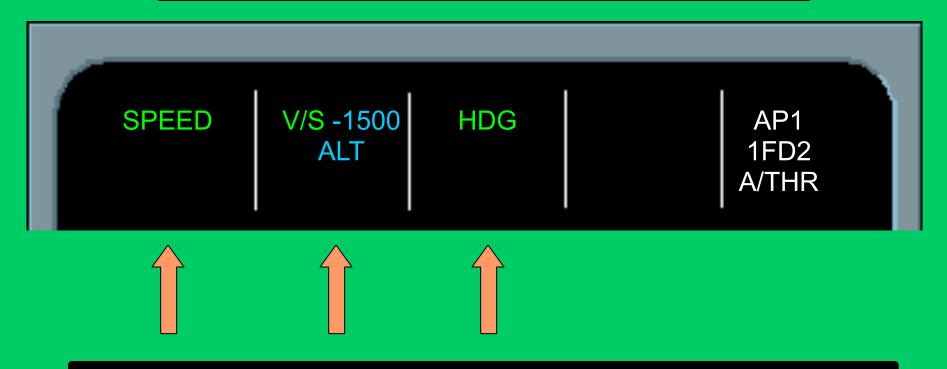
During Managed Descent, the HDG knob is pulled. THR IDLE changes to SPEED, DES to V/S on current V/S. NAV to HDG. Point to note, all three columns change.
