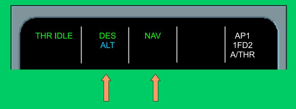
First push the HDG knob, and then push the ALT knob. When HDG is pushed, HDG changes to NAV (limitations??). When ALT knob is pushed, OP DES changes to DES.
