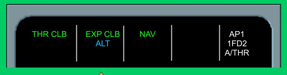
When EXPED P/B on FCU is pushed, EXP CLB in Green. Target speed GREEN DOT.
