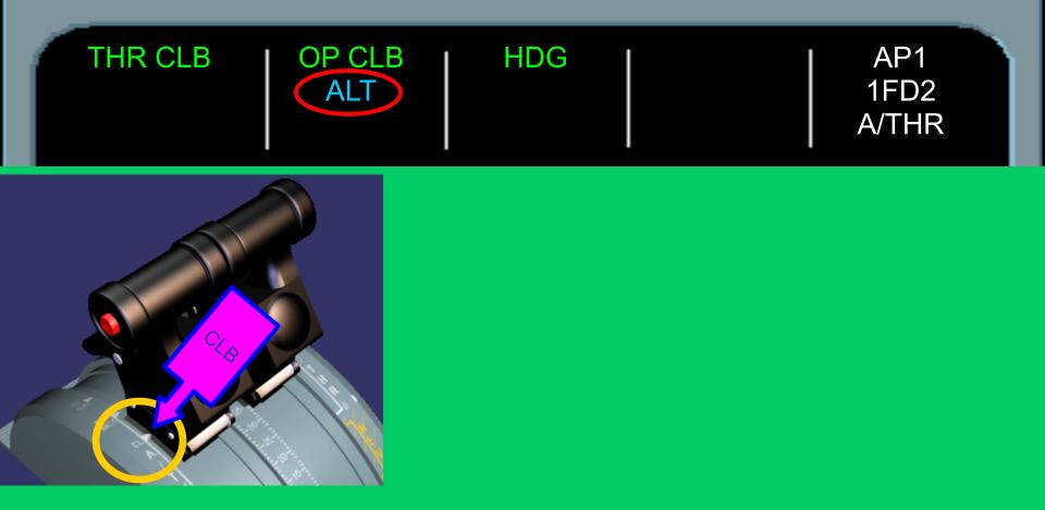
At GA Acceleration Altitude, Thrust Lever is in CLB detent. Alt armed (In Blue). Engagement of HDG means we are under Radar HDG. OP CLB as we are in HDG.
