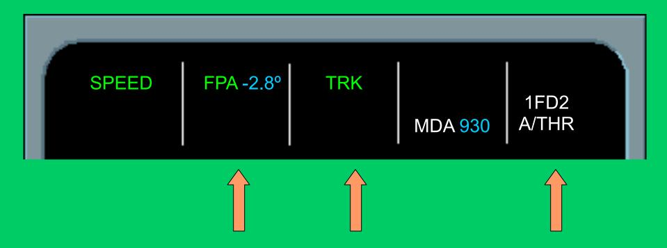
When A/P is disconnected or happens automatically at MDA -50 feet or at 400 ft if no MDA entered. The FDs revert to basic modes (HDG-V/S or TRK-FPA)
