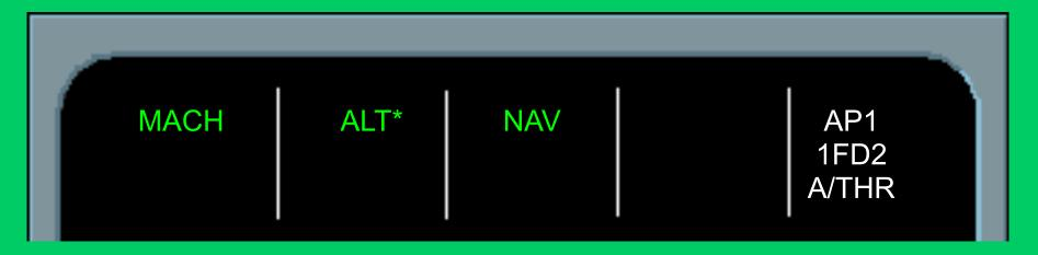
At ALT\* engagement, EXEP CLB automatically disengages.
