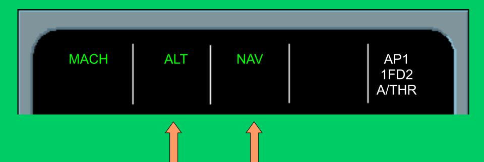
Above (ALT in Green) shows that the aircraft has leveled off at altitude below the FMGC entered altitude.
