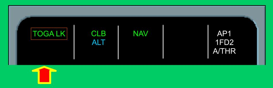
Auto Thrust active and TOGA Thrust is locked. "Alpha Floor" conditions are no more met. Pilot must disconnect A/THR.
