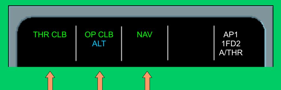
Pull the ALT knob, SPEED changes into THR CLB, V/S into OP CLB and no change in NAV.
