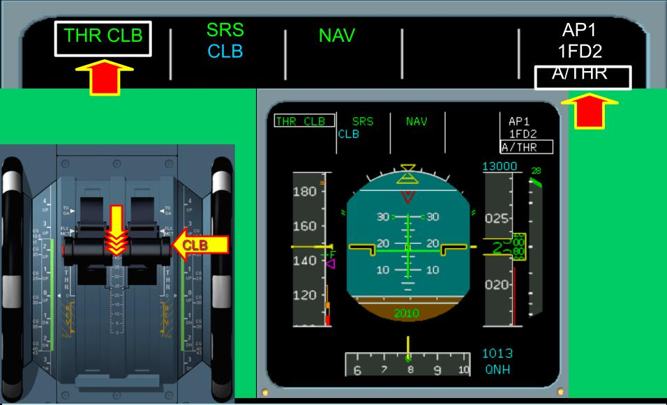
When Thrust Lever is set to Climb Detent, THR CLB in Green, and Auto Thrust in White. (Both in Engaged Mode)
