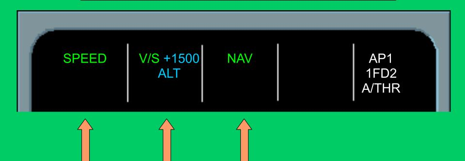
THR CLB changes to SPEED, CLB becomes the current V/S. Thrust may reduce to maintain the current V/S (priority) & then the desired speed. NAV remains as it is.
