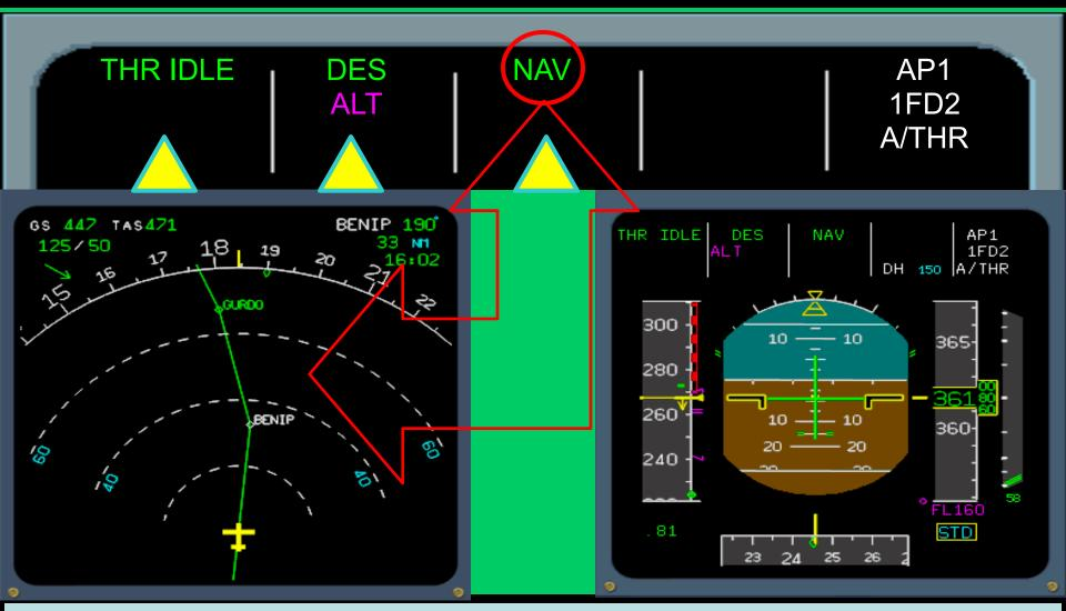
During Managed Descent, 2<sup>nd</sup> column DES means vertical constraints will be met. Thrust can be THR IDLE or MACH/SPEED. NAV means lateral Flt Plan is being followed.
