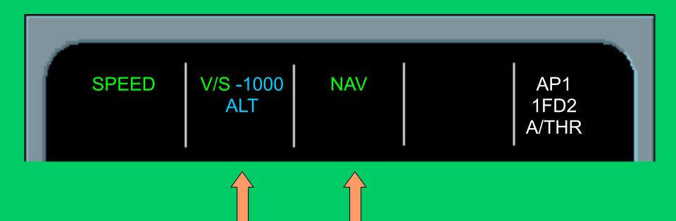
Either select a vertical speed say 1000 ft/min, to go down to the selected altitude on FCU or...
