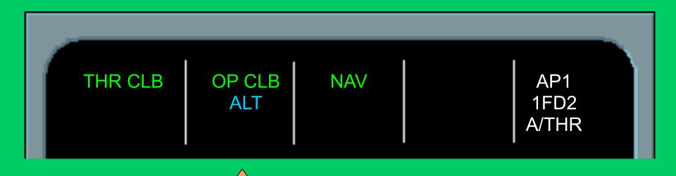
To revert to Open Climb, Pull the ALT selector knob on FCU, OPEN CLIMB mode will engage.
