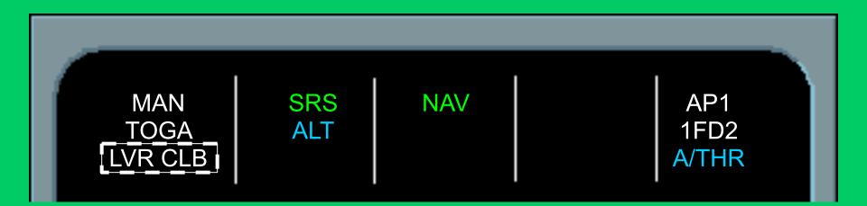
At Thrust Reduction Altitude, LVR CLB flashes. Alt armed (In Blue). Engagement of NAV means we are following Missed Approach Procedure.
