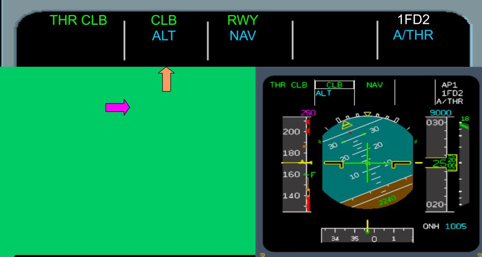
In case you want to revert to the Managed Speed, push the Speed knob on FCU. On PFD speed target goes to 250 Kts shown as a Managed Magenta ( ). CLB remaires the engaged mode and ALT remains armed in Blue.
