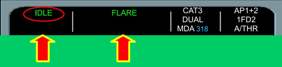
At 30 feet AGL FLARE remains Green. IDLE on the Auto Thrust Column.
