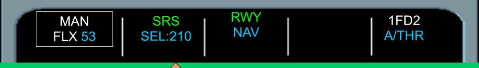
As soon as the thrust lever is set in FLEX/TOGA detent, Pre Selected Climb Speed 210 Kts becomes armed (in Blue) and <u>SEL:210</u> is displayed on FMA. This Pre Selected Climb Speed 210 Kts was entered in the FMGC (PERF Climb Page). SRS is engaged in vertical mode.
