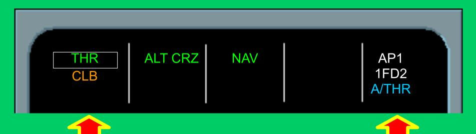
In some aircraft, (AP-BGU & BGV) both thrust levers are moved ahead of Climb Detent, "THR" in Green steady with a white box, with "CLB" in amber flashing. Advising Pilot to Set Thrust Lever to Climb Detent. A/THR becomes BLUE i.e. armed.
