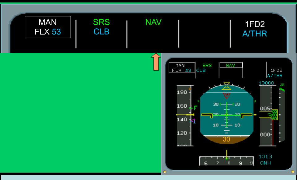
If NAV is armed, engages automatically at 30 Feet RA.
