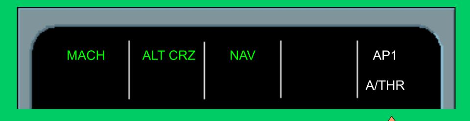
Normal Cruise conditions. Both FDs selected OFF. AP-1 is ON. No change in other FMA columns. The last Column reads AP1. FD indications blank.
