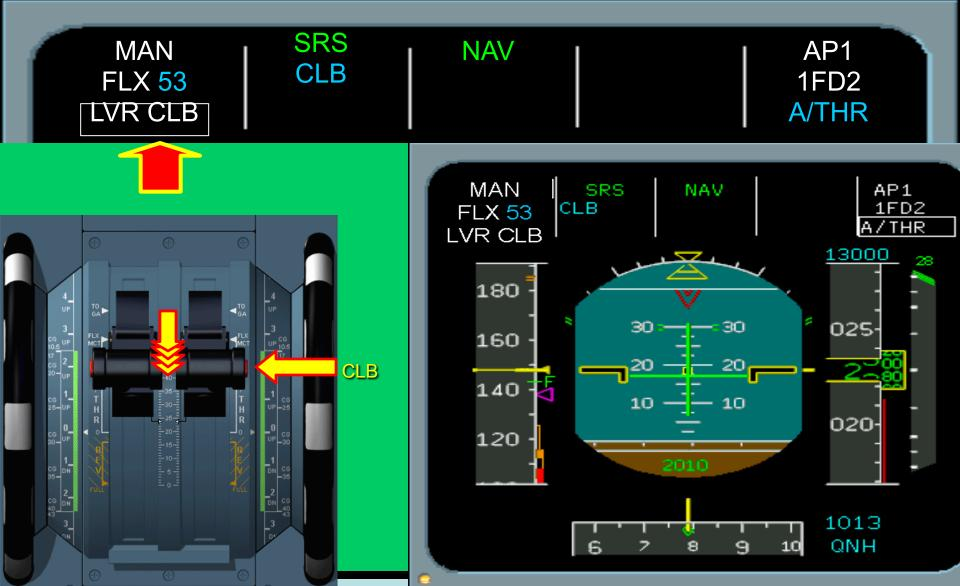
At Thrust Reduction Altitude "LVR CLB" Flashes. Advising Pilot to Set Thrust Lever to Climb Detent
