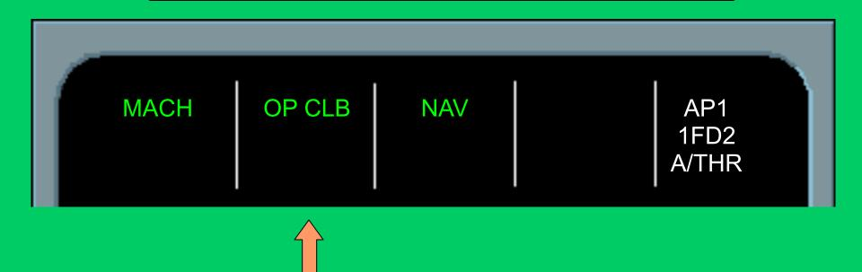
Pull the ALT knob on the FCU to engage Open Climb. You can also adjust the V/S to reach the desired level.
