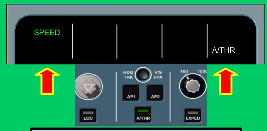
Normal Cruise conditions. Both FDs OFF. A/P is OFF. A/THR goes in SPEED mode. Lateral & Vertical column become blank. AP & FD indications go OFF.
