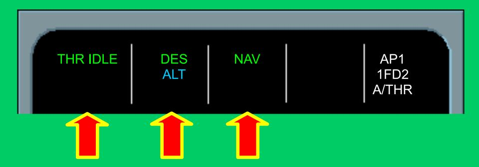
During Managed Descent, 2<sup>nd</sup> column DES means vertical constraints will be met. VDEV will be kept zero on PROG Page. Thrust can be THR IDLE or MACH/SPEED. NAV means lateral Flt Plan is being followed.
