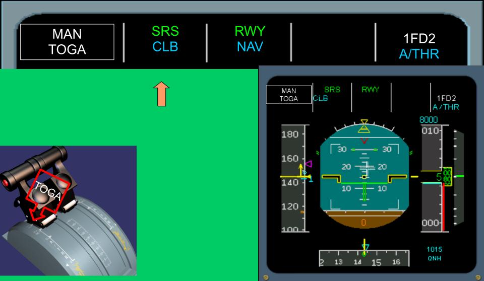
When thrust lever is set in FLEX/TOGA detent. SRS engages in pitch mode to give V2 to V2+10 Kts. Climb armed (in Blue). If V2 not entered in the FMGC (PERF Take Off Page). SRS does not engage.
