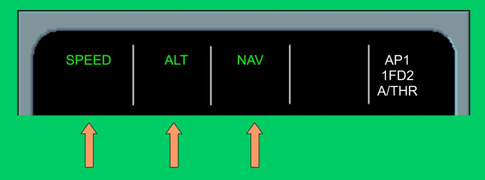
Initial aircraft configuration. Managed mode for ILS (below the Glide Slope).
