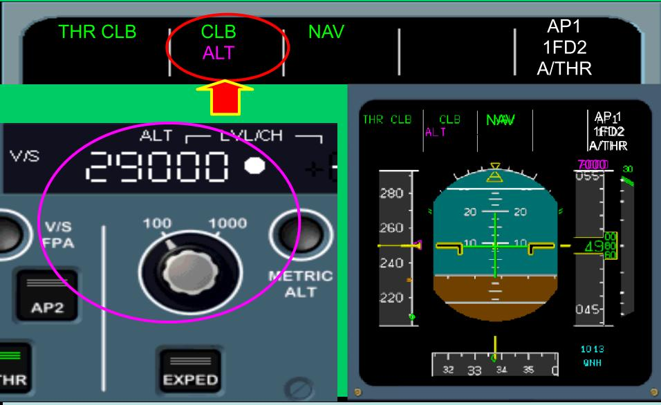
There is an Altitude Constraint at, say FL 070. ALT (in magenta) is the FMGC constraint. FCU ALT set at FL-290.
