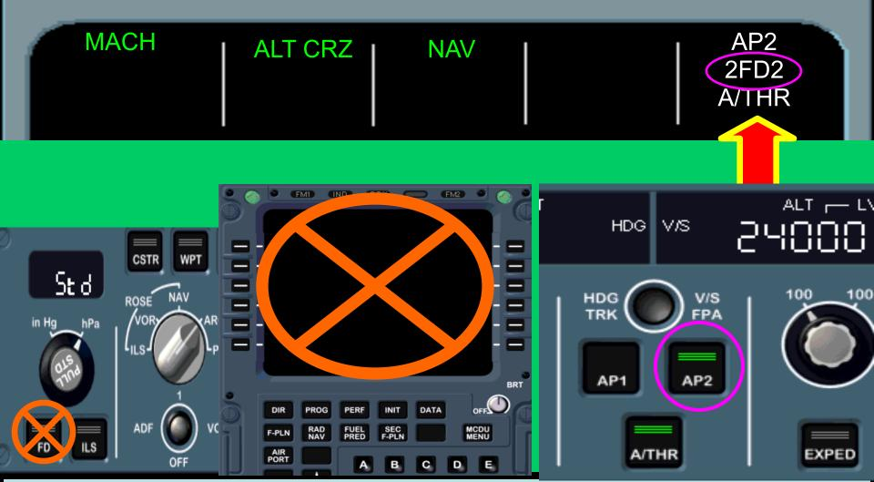
One FD fails or One FMGC fails or is not valid. AP2 is connected. Both FMAs show 2FD2. Both FDs are ON. FD lights on the FMA are ON.
