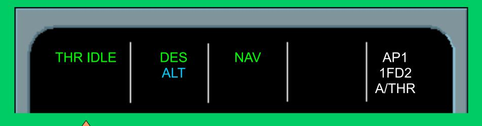
SPEED changes to THR IDLE (as you are above profile), you need to use S/B to increase ROD to get back on profile. As you reach the correct profile, S/B will flash in amber in Memo (E/ WD on Upper ECAM). Retract S/B.
