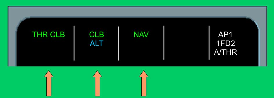
Push the ALT knob, SPEED changes into THR CLB, V/S into CLB and NAV remains as it is.
