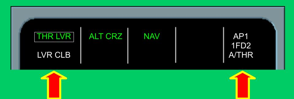
If one Thrust Lever (AP-BRJ) is moved ahead of the Climb Detent, THR LVR in Green with a white box. "LVR CLB" flashes in white. Set the Thrust Lever in climb detent. A/THR remains Active (White).
