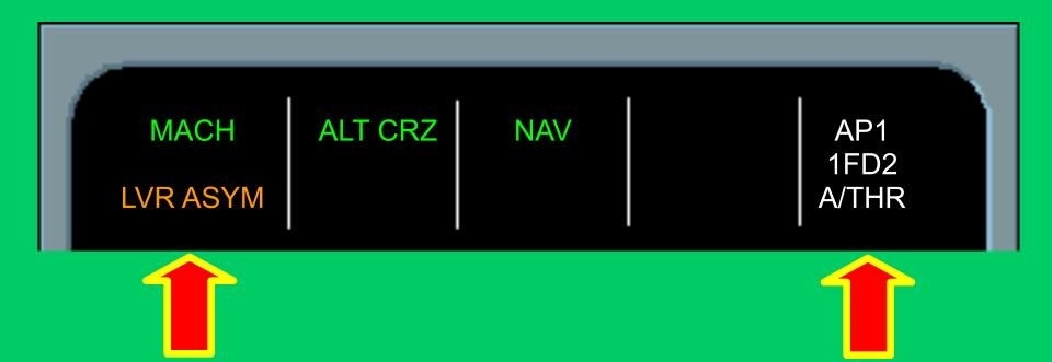
In a Normal Cruise (AP-BRJ) if one Thrust Lever is moved below the Climb Detent LVR ASYM in steady amber. Set the Thrust Lever in climb detent. A/THR is Active (White).
