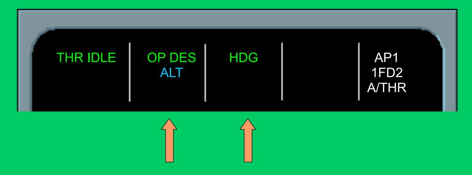
Thrust will be THR IDLE. The speed triangle on the speed tape is managed magenta ( ) lowever, during managed descent it is an open bracket with a speed range of ± 20 Kts.
