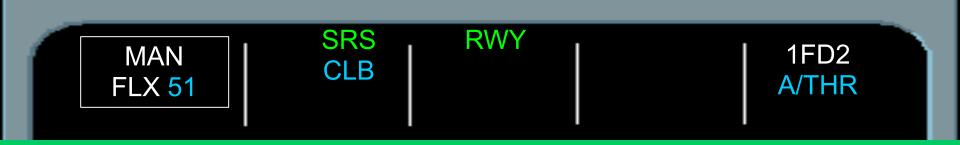
With HDG pre set say HDG 143°, Lateral Column which was blank, changes to RWY as thrust lever is set in FLEX/ TOGA detent. RWY engages only if Runway is ILS equipped and the ILS signal is valid.
