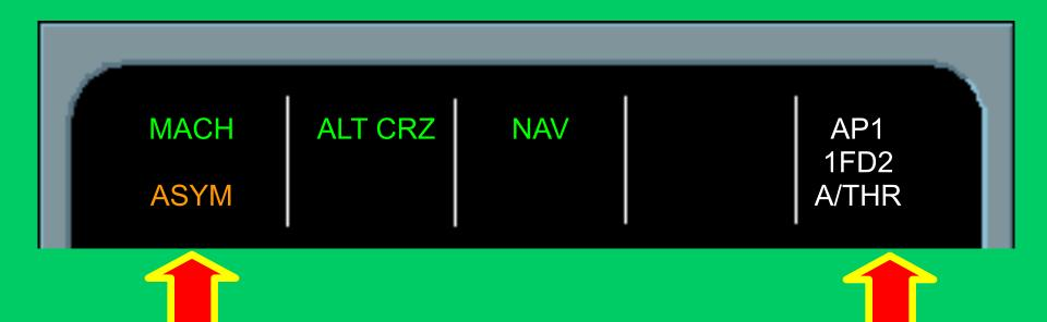
In some aircraft (AP-BGU & AP-BGV) if one Thrust Lever is moved below the Climb Detent ASYM in steady amber. Set the Thrust Lever in climb detent. A/THR remains Active (White).
