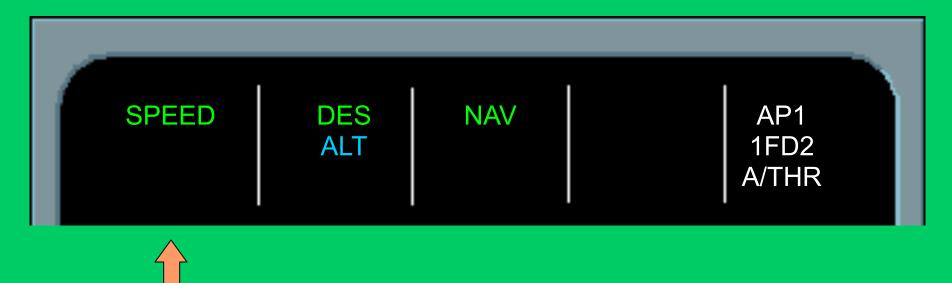
THR IDLE changes to SPEED (as you are below profile), thrust added to correct the profile. DES mode keeps the aircraft on the profile; VDEV zero on the PROG Page.
