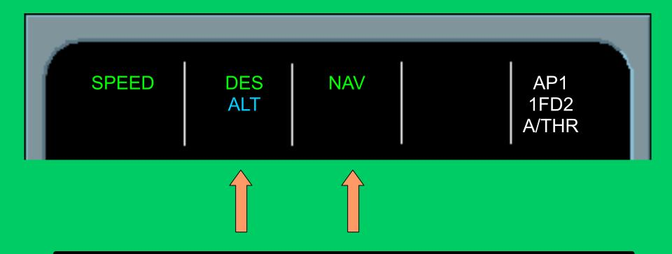
THR IDLE changes to SPEED. Thrust is added to get the higher speed. As DES is engaged, the VDEV remains zero. The speed triangle on the speed tape is selected blue ( ).
