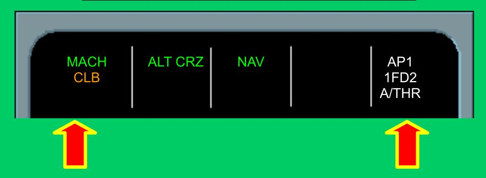
In some aircraft (AP-BGU & BGV), when both thrust levers are moved below Climb Detent, "CLB" in Amber Flashes. Advising Pilot to Set Thrust Lever to Climb Detent. A/THR no change. No M/Caution or ECAM Warning.
