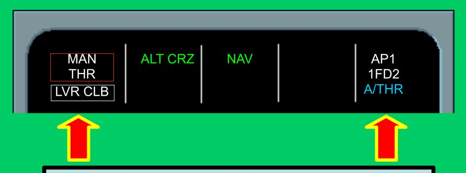
When both thrust levers (AP-BRJ) are moved ahead of Climb Detent, "MAN THR" in steady white with Amber box, and "LVR CLB" flashing. Advising Pilot to Set Thrust Lever to Climb Detent. A/THR becomes BLUE i.e. armed.
