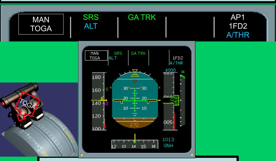
Go Around SRS in pitch mode. Alt armed (In Blue) to the GA Altitude
