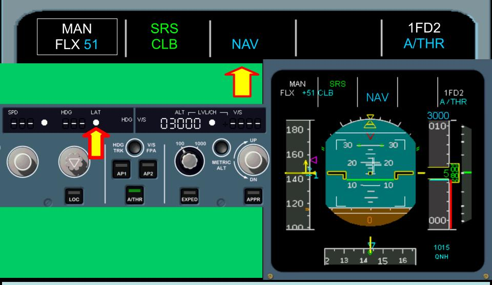
When thrust lever is set in FLEX/TOGA detent, RWY not displayed, if no ILS on that Runway or ILS signal Not Available. Navigation armed (In Blue)
