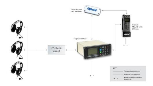
FIGURE 1: STANDARD INSTALLATION
