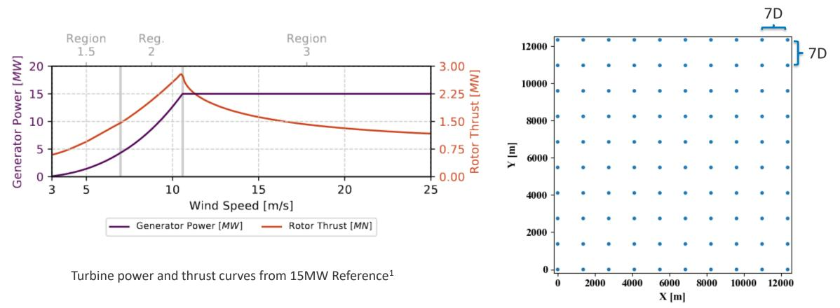
Reference plant layout for 2022 (10-MW turbine). Dot size = 1D
