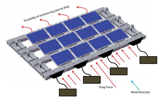
Figure 24: Schematic of drag forces developed in floating solar PV plant
