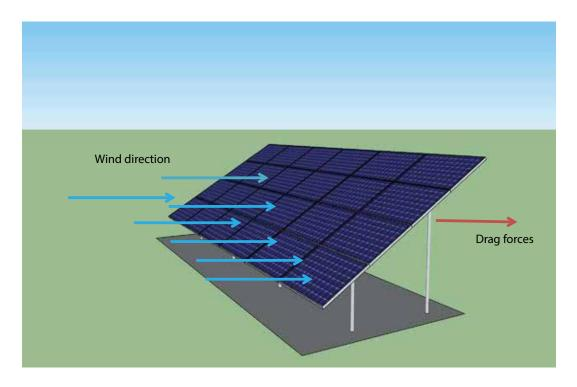
Figure 23: Drag forces in ground-mounted solar PV (only for representational purpose)
