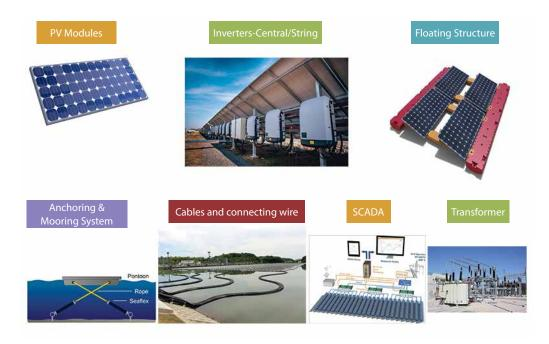
Figure 2: Major components of floating solar PV
