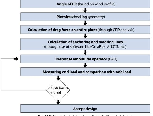
Chart 18: A flow chart of steps in floating solar PV project design Source: TERI's analysis
