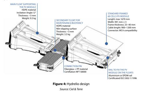
countries, accounting for more than 300 MWp of installed capacity. Hydrelio floats are made of HDPE and connection pins are made of polypropylene combined with fiberglass. The floats are manufactured by blow molding and pins are made from injection molding.
