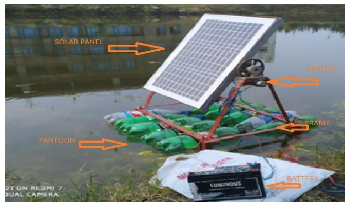
Fig-2: Floating photovoltaic solar power plant
