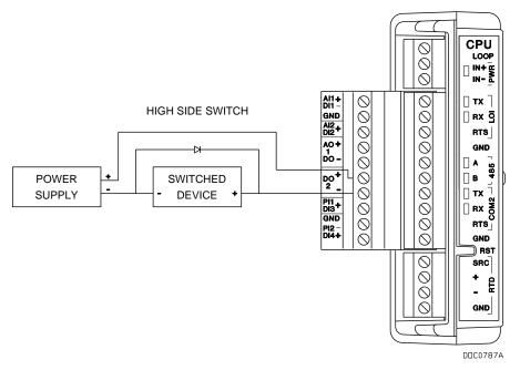
Figure 4-14. Discrete Output Wiring - High Side Switch (on CPU Module)
