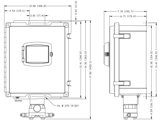
Figure 1-5. Polycarbonate enclosure with a DVS module
