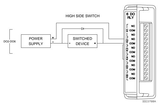
Figure 4-15. Discrete Output Relay Module Wiring (High Side Switch)
