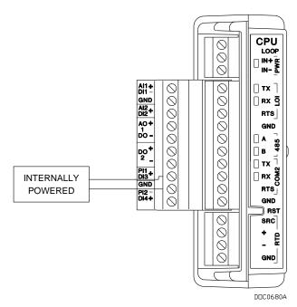
Figure 4-17. Pulse Input Wiring (on CPU Module)
