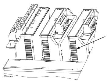
Figure 4-3. Ridged Edges on Modules
