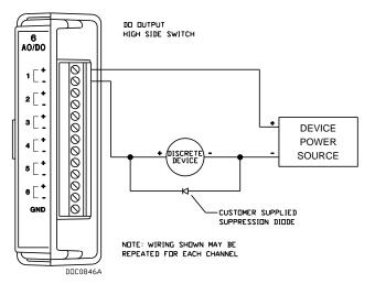
Figure 4-23. Discrete Output High Side Switch Wiring
