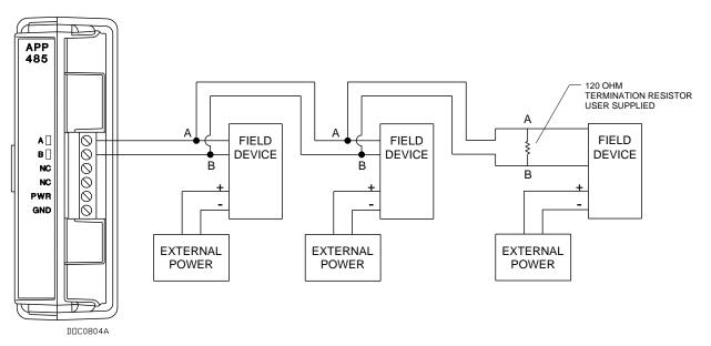
Figure 4-19. Application Module Wiring to Multiple Field Devices
