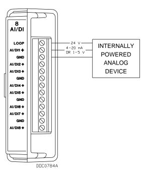
Figure 4-9. AI Wiring (Internal Power)
