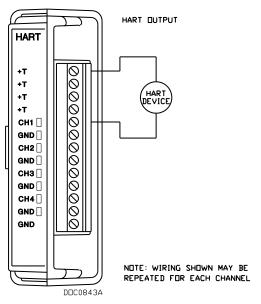
Figure 4-27. HART Output Wiring
