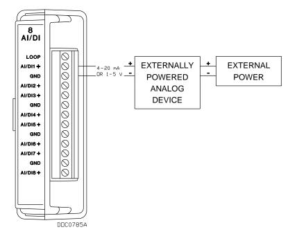
Figure 4-10. AI Wiring (External Power)
