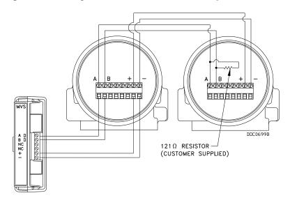
Figure 6-3. MVS Multi-Drop Configuration with Two Transmitters
