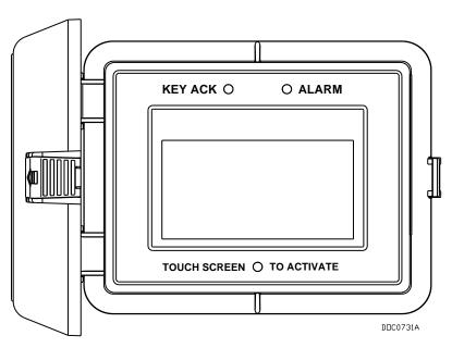
Figure 5-4. Liquid Crystal Display ("Touchpad")
