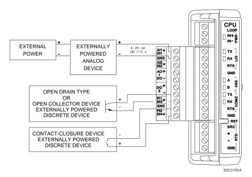
Figure 4-6. Loop Output Power for the CPU Module's Optional I/O Assembly
