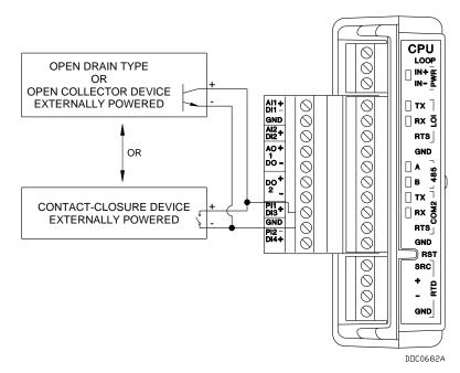
Figure 4-12. Discrete Input Wiring (on CPU Module)
