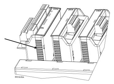
Figure 2-8. Ridged Edges on CPU Module
