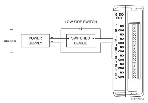
Figure 4-16. Discrete Output Relay Module Wiring (Low Side Switch)
