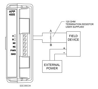
Figure 4-18. Application Module Wiring to Single Field Device
