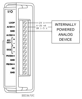
Figure 4-7. Loop Output Power for the I/O Module
