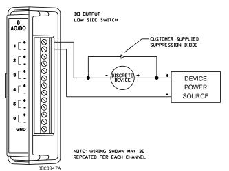
Figure 4-24.. Discrete Output Low Side Switch Wiring
