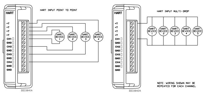
Figure 4-25. HART Input Point-to-Point Wiring
