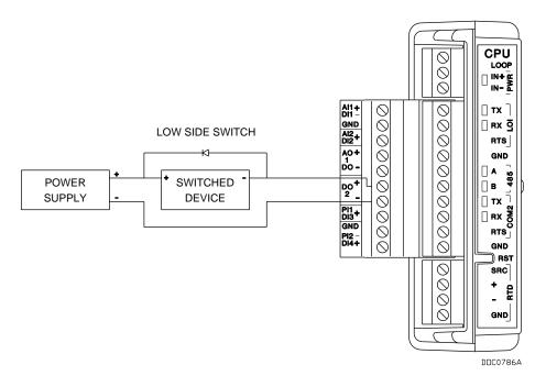
Figure 4-13. Discrete Output Wiring - Low Side Switch (on CPU Module)
