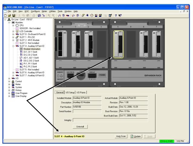
**Note:** *Figure 4-5* shows the default values for an I/O module.
