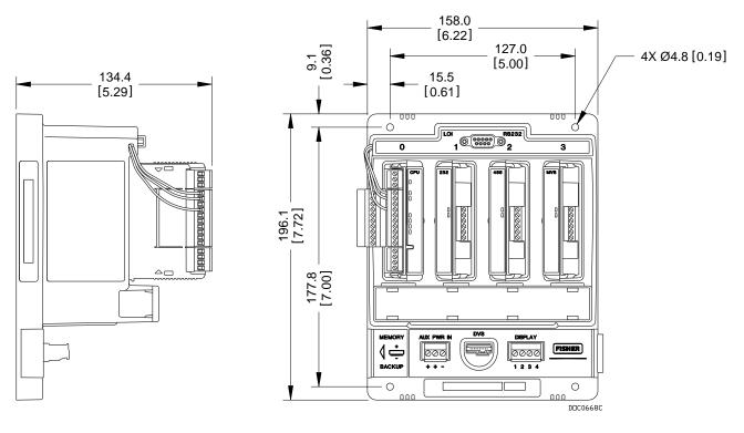
Figure 2-1. Side and Front View of FloBoss 107 Base Unit
