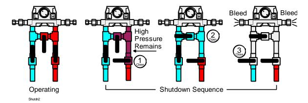
Figure 7-3. DVS Depressurization
