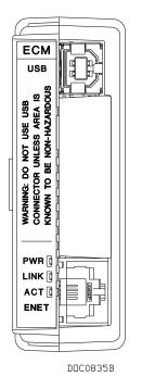
Figure 5-6. Enhanced Communication Module (ECM)
