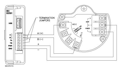
Figure 4-31. FB107 IEC 62591 Module Power and Data Wiring to Field Link
