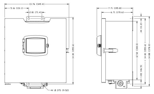
Figure 1-6. Steel enclosure with a PIM module
