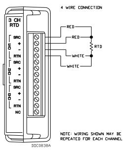
Figure 4-30. 4-Wire Connection Wiring
