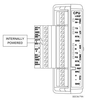
Figure 4-11. Analog Output Wiring (on CPU Module)
