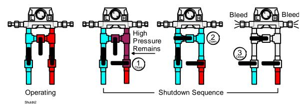
Figure 7-2. MVS Depressurization
