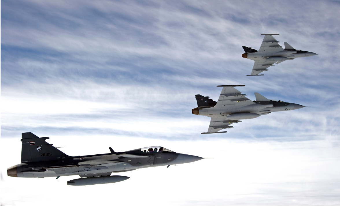
Figure 2.3: Three military Saab Gripen fighters flying in tight formation. The line resembles half a V, and the wind resistance is reduced for all but the first plane.
