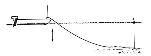
Figure 5:13—Anchor Buoy
