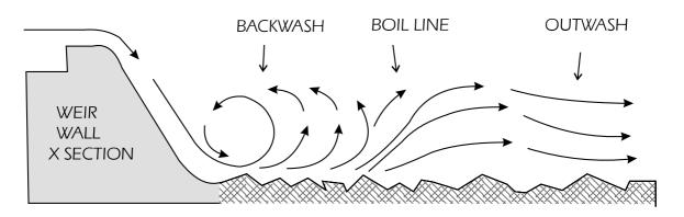
Figure 3:11—Water Currents below Weirs (elevation view)
