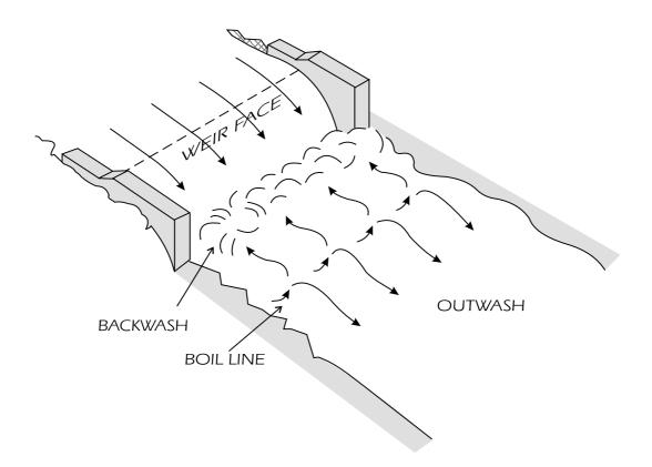
Figure 3:10—Water Currents below Weirs (plan view)
