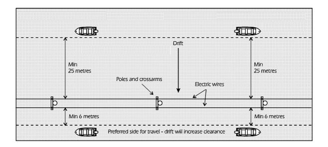
Figure 3:15—Travel Alongside a Wooden Power Line where there is Lateral Drift (not to scale)
