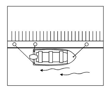
Figure 9:4—Securing Alongside
