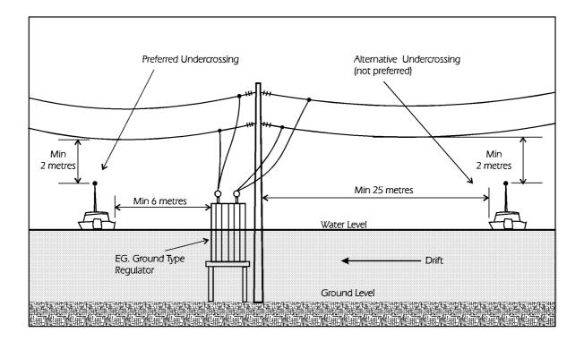
Figure 3:13—Undercrossing Near Ground Structures—Wooden Pole Lines (not to scale)
