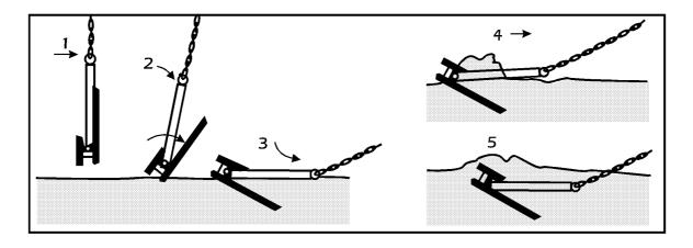
Figure 5:17—How the Danforth Anchor Holds
