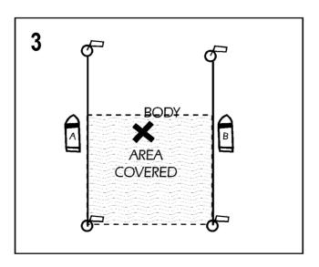
Figure 11:10—Dragging Boat to Boat
