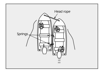
Figure 9:9—Barge Towing
