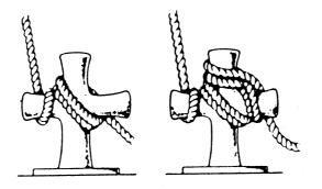
Figure 5:8—Belaying a Rope to a Bollard
