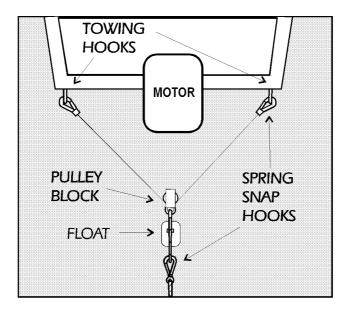
Figure 9:6—Pulley Bridle
