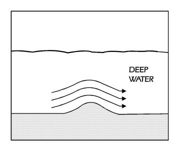
If the water is shallower the bump caused by the water being forced upwards may appear as a wave on the surface. (See Figure 3:3).
