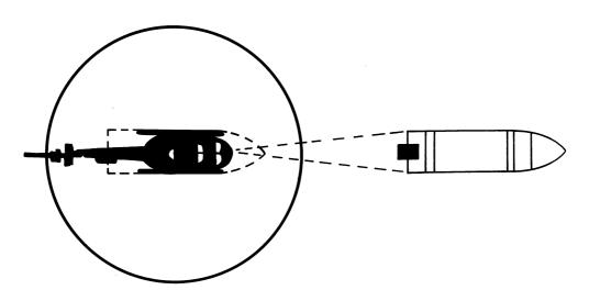
Figure 9:11—Helicopter Winching Position
