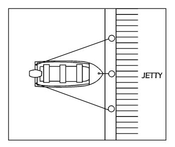
Figure 9:5—Secured 'Bow on' by Quarter Lines
