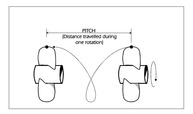
Figure 7:7—Propeller Pitch
