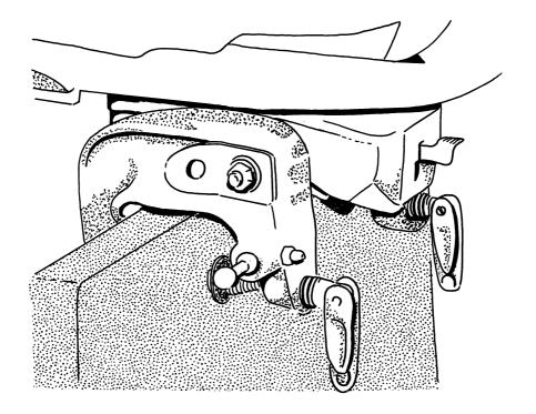
Figure 7:6—Motor Mounted and Clamped to Transom
