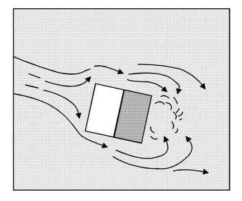
Figure 3:7—Currents around a Structure
