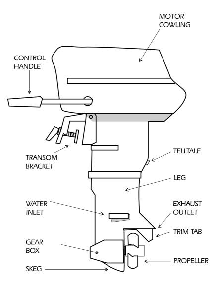
Figure 7:1—Parts of an Outboard Motor
