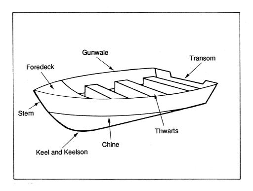
Figure 5:3—Boat Hull Parts
