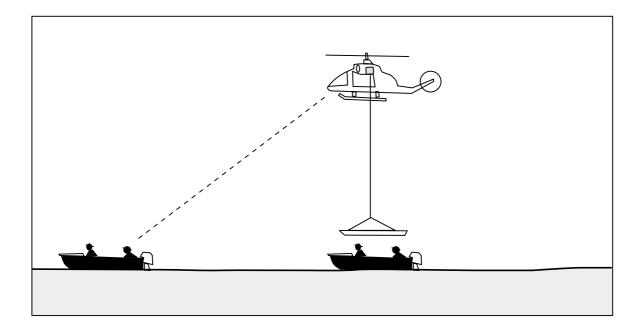
Figure 9:12—Helicopter Winching Position
