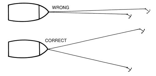
Figure 5:14—Using Two Anchors
