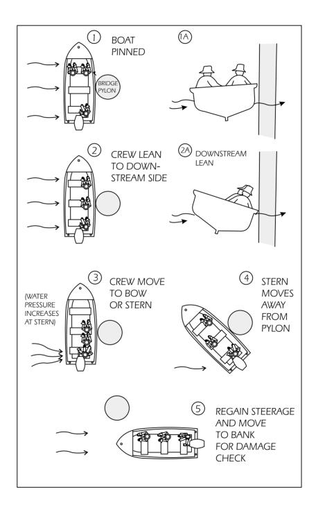
Figure 9A:2—Boat Pinning Drill
