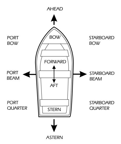
Figure 5:4—Terms of Boat Direction and Location
