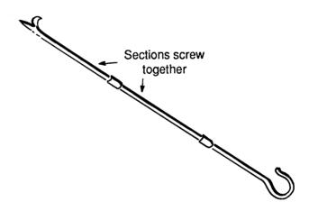
Figure 11:3—Pike/Pole Iron for Probing or Grappling
