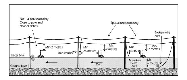
Figure 3:14—Undercrossing Wooden Pole Lines (not to scale)
