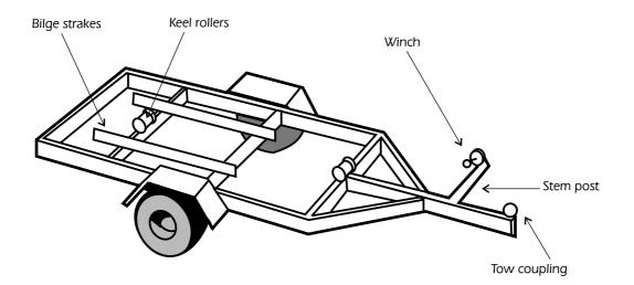
Figure 6:1—FRB Trailer with Bilge Strakes
