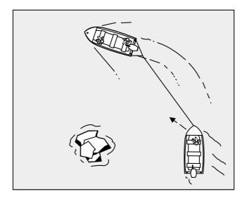
Figure 9:8—Towing with a Bridle
