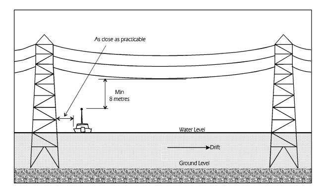
Figure 3:17—Undercrossing Steel Power Lines (not to scale)
