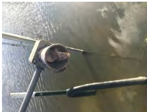
Figure 4. Example of spider webs in the cone of an ultrasonic sensor.
