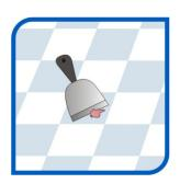
3. Depending on the size of the cleaning area, vacuum using an OGS-approved backpack or other canister-type vacuum. Beginning at the furthest point of the work area, vacuum using an overlapping back-and-forth motion.. Make sure the corners and edges of the floor are clean.
