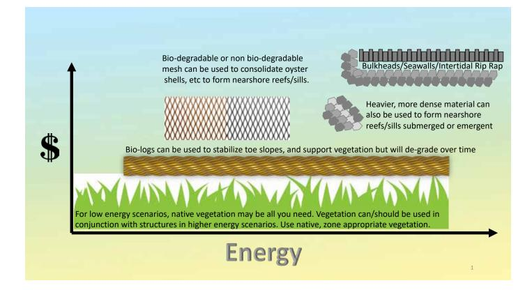
This graph illustrates how wave energy increases the extent of stabilization measures and cost associated with projects. In NW Florida, we utilize *Spartina alterniflora* as our main intertidal grass, which has a fairly specific tolerance to wave energy. If one can determine that a shoreline experiences an energy climate that exceeds that threshold, typically done by observation and/or online evaluation, then it is appropriate to consider installing coir logs or a reef structure.
