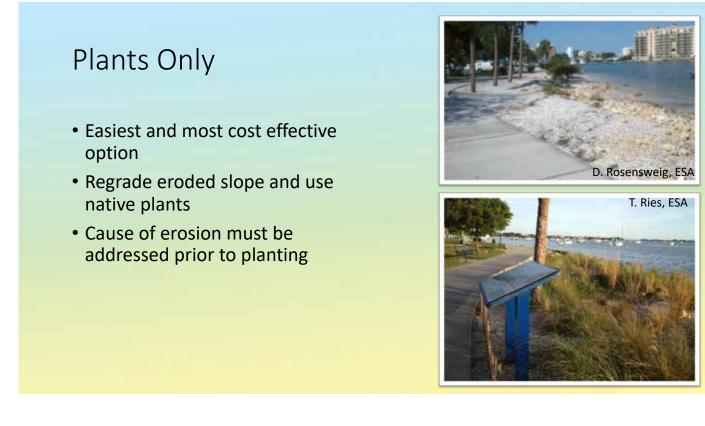
Planted Shoreline - the easiest and least cost expensive option is just regrading the eroded slope and planting with native vegetation, which worked at this site in Sarasota Bay; however, if there was an eroded bank, the cause of the erosion **must** be addressed (e.g. minimum wake zone enacted or wave energy protection installed) before just installing plants along the shoreline.
