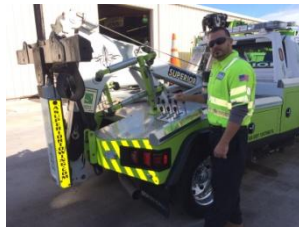
A Superior operator Yanir Zarka wearing his ANSI 3 safety apparel stands with his truck marked with highly reflective lettering to create a larger safety footprint and reflective tape on both the rear and sides.
