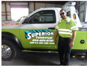
A Superior operator Yanir Zarka wearing his ANSI 3 safety apparel stands with his truck marked with highly reflective lettering to create a larger safety footprint and reflective tape on both the rear and sides.
