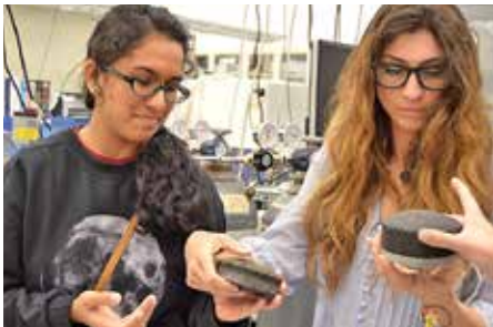
Sakhee Bhure, astronomy and astrophysics major, and Victoria Jenne, astrobiology major, hold regolith simulant tested for heat shield use at NASA's Swamp Works.
