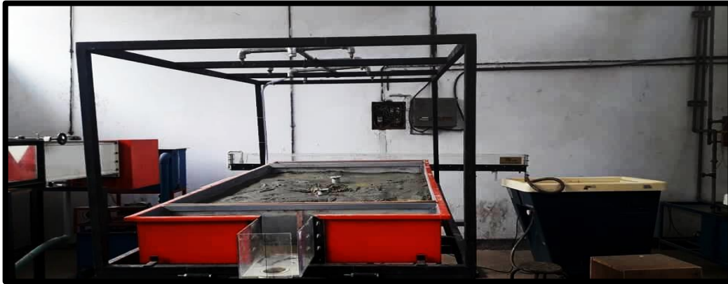
Figure 3: The sand catchment preparation in the simulator at hydraulic laboratory
