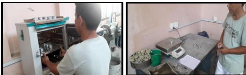
Figure 5: Moisture content determination (soil laboratory, purwanchal campus Dharan)
