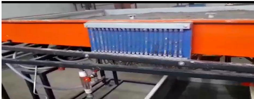
Figure 4: Manometer set for pressure measurement developed in the soil due to rainfall
