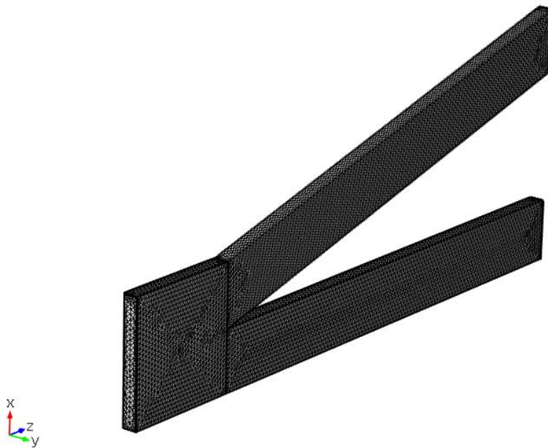
Figure 10. Resulting geometry including mesh used for evaluation of gravity and Reynolds number effects on flow distribution.
