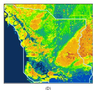
Figure 2. Landsat Thematic Mapper vegetation image (A), model vegetation grid (B), resistance-coefficient values assigned to vegetation (C), and model resistance-coefficient grid (D).
