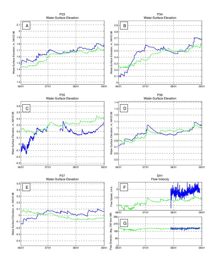
Figure 4. Simulated (dashed green line) and measured (solid blue line) water-surface elevations at sites P33 (A), P34 (B), P35 (C), P36 (D), and P37 (E) and flow speeds (F) and directions (G) at site SH1.
