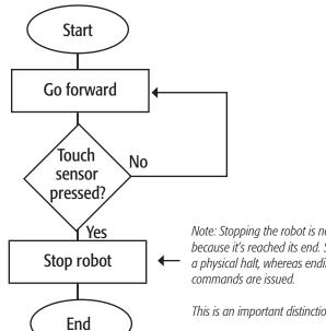
Note: Stopping the robot is not the same as the program stopping because it's reached its end. Stopping the robot means bringing it to a physical halt, whereas ending the program simply means no more
