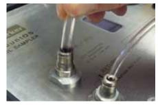
Low Pressure Connection Connect INLET (Ø 6mm) hose
