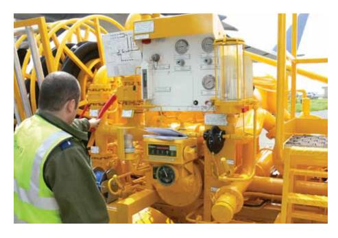
This application shows uploading fuel into an aircraft with the icountPD in use to monitor as a 'go/no go' device.
