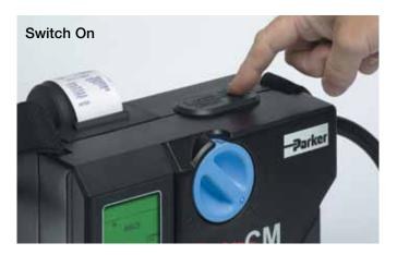
Operating the Parker icountLaserCM is as simple as pressing the start button and turning the dial. The test procedure is automatic and in the case of the icountLaserCM takes no more than 2 minutes to complete.
