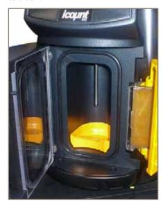
Fig 4. The IBS2 oil sampling probe automatically lowers into the bottle once the test begins.
