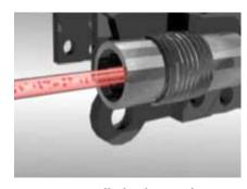
Fig 1. A controlled column of contaminated fluid enters the laser optical scanning chamber, which is designed to ensure balanced flow and fluid distribution for consistent results.
