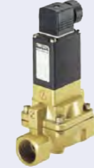
Type 5282 2/2 way, Servo Assist Solenoid Valves With Separating Diaphragm Isolating Media From Solenoid System, Opening and Closing Time Adjustment and Manual Override Standard Normally closed or normally open function
