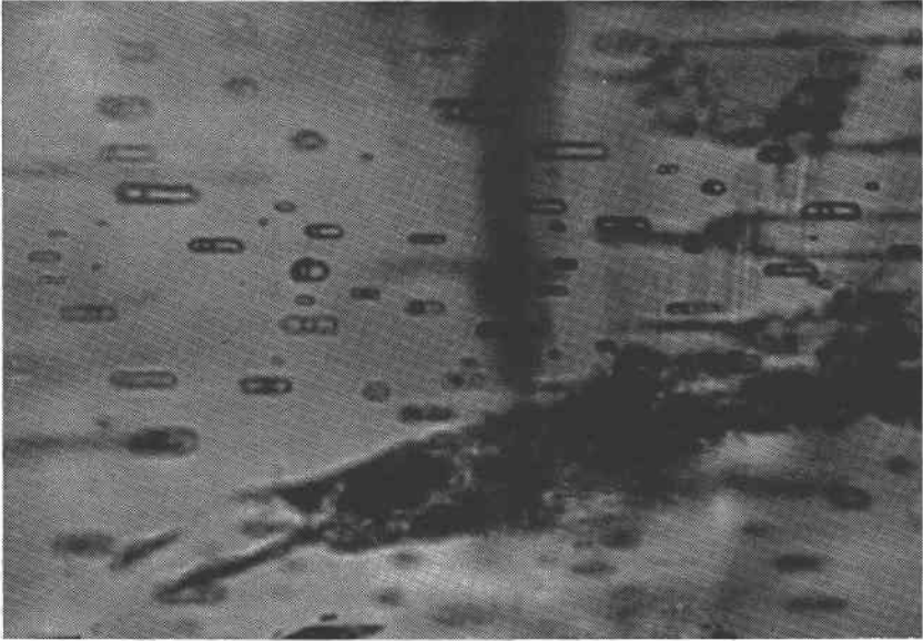
FIG. 3. Negative crystal inclusions in beryl, oriented parallel to the c axis. Selden east pegmatite. \times 200 .
