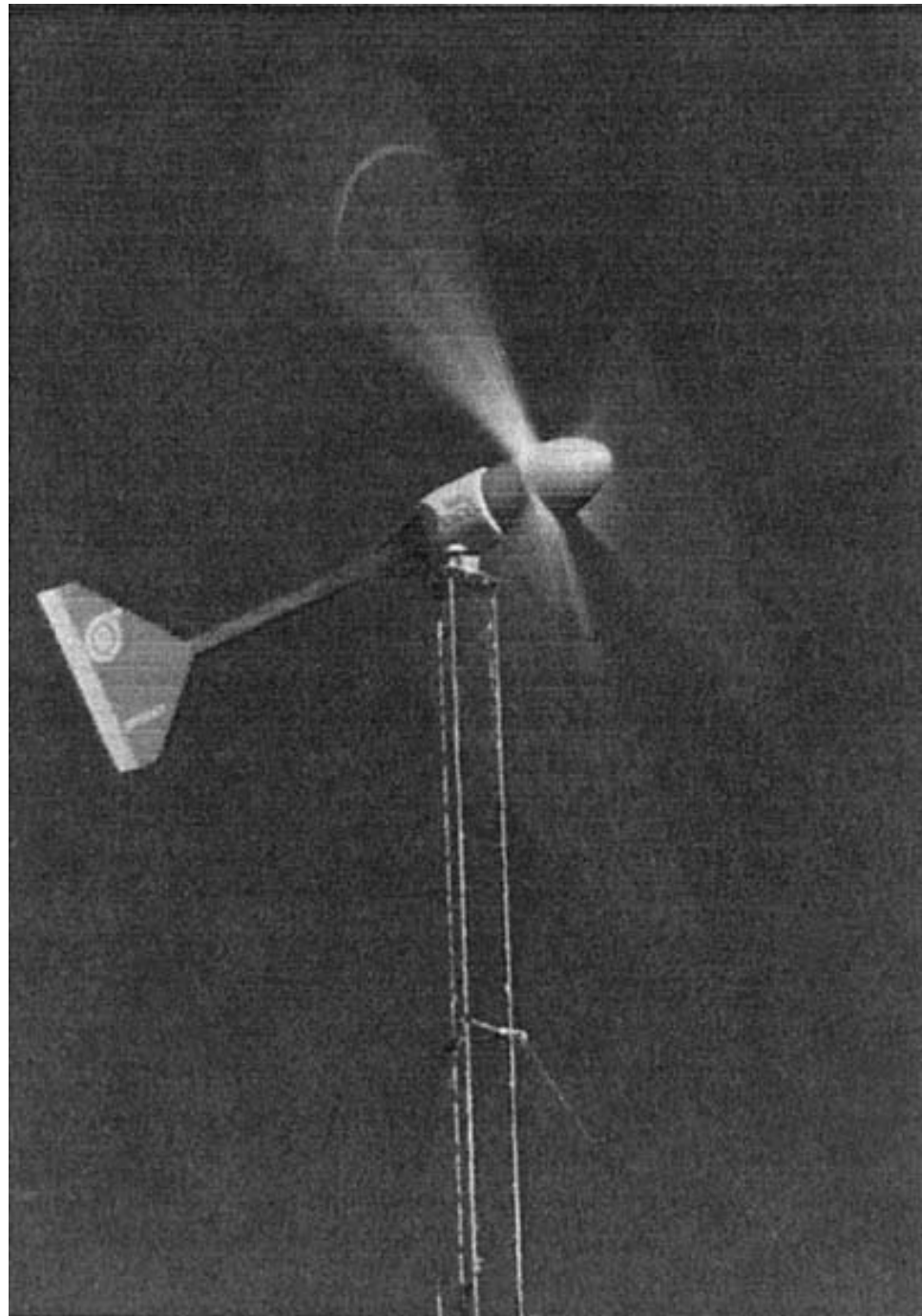
FIG. 10.4. (b) The Bergey Excel-S, three-bladed, 7 m diameter wind turbine, rated at 10 kW at wind speed of 13 m/s. (With permission of Bergey Windpower Company.)
