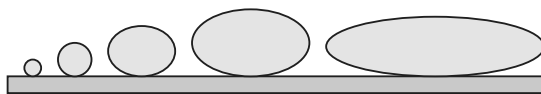
Fig. 1.9 The larger droplets are flatter because gravity is becoming more important than surface tension.
