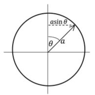
The second way is a purely geometric argument. Consider the following schematic. To find the dostamce between the surface and the axis of rotation, we see that we need to a factor of  $a\sin\theta$  such that  $u_{\phi} = a\Omega \sin\theta$  at r = a.
