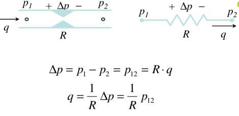
Orifices, valves, nozzles and friction in pipes can be modeled as fluid resistors.
