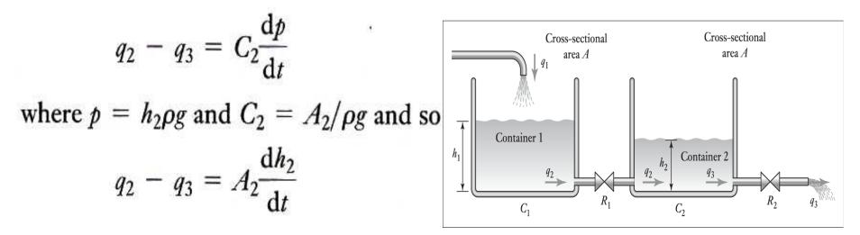
The rate at which liquid leaves the container  $q_3$  equals the rate at which it leaves the valve  $R_2$ . Thus for the resistor,
