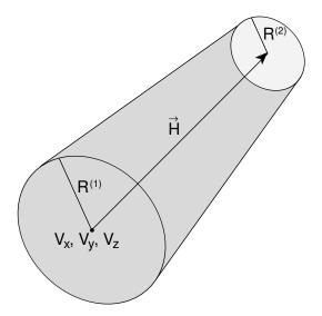
Fig. 8.6: Truncated Right Angle Cone (TRC)
