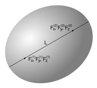
Fig. 8.7: Ellipsoid of Revolution (ELL)
