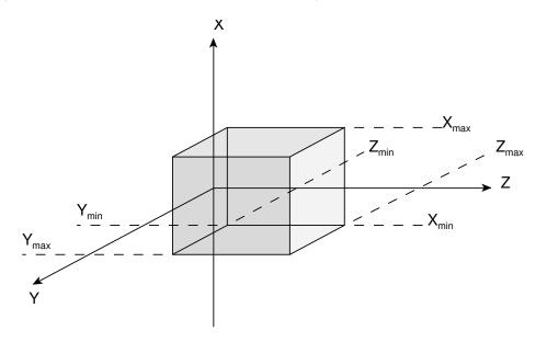
Fig. 8.1: Rectangular Parallelepiped (RPP)
