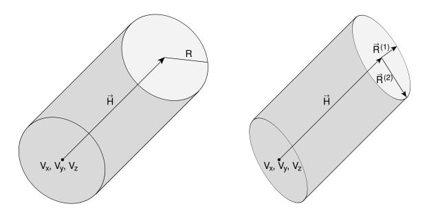
Fig. 8.4: Right Circular Cylinder (RCC)
