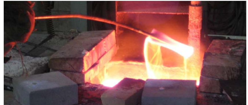
Molten Chloride Salt Metallic Heat Treatment Bath (1100°C)
