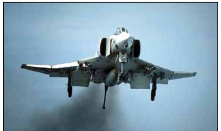
Gear down, flaps down, hook down, harness locked...Here I come, 17 tons @ 145 knots
