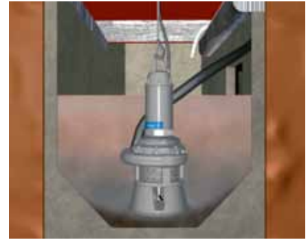
Agitator for coarser slurries.
