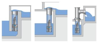
Installation is steel, plastic or concrete column lifting to an open channel. No check valve is required.
