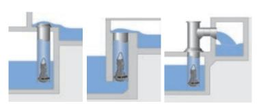
Installation in steel, plastic or concrete column lifting to an open channel. No check valve is required.
