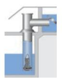
With submerged outlet and flap valve.
