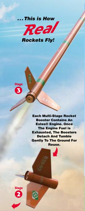
**Multi-Stage Rocket** Flight Sequence **STREAMER** RECOVERY **BOOSTER SEPARATES** AND TUMBLES THIRD STAGE, **ROCKET ENGINE IGNITES BOOSTER SEPARATES** AND TUMBLES SECOND STAGE. **BOOSTER IGNITES** FIRST STAGE, **BOOSTER IGNITES** LIFTOFF!
