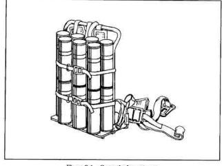
Figure 8-4. Cargo tie-down straps.
