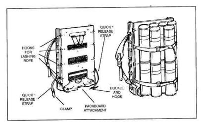
Figure 8-7. Typical packboard load.
