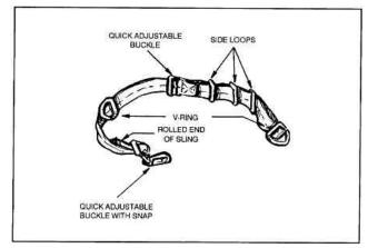
Figure 8-5. Universal load-carrying sling.
