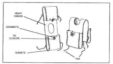
Figure 8-10. Locally fabricated load-carrying vest.
