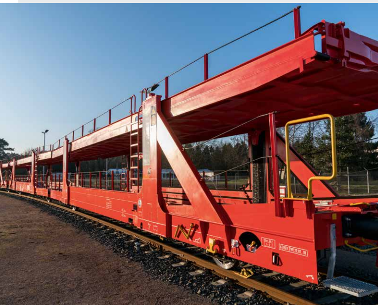
— The wagon is 33 m long and equipped with telematics and a flexible load securing system.
