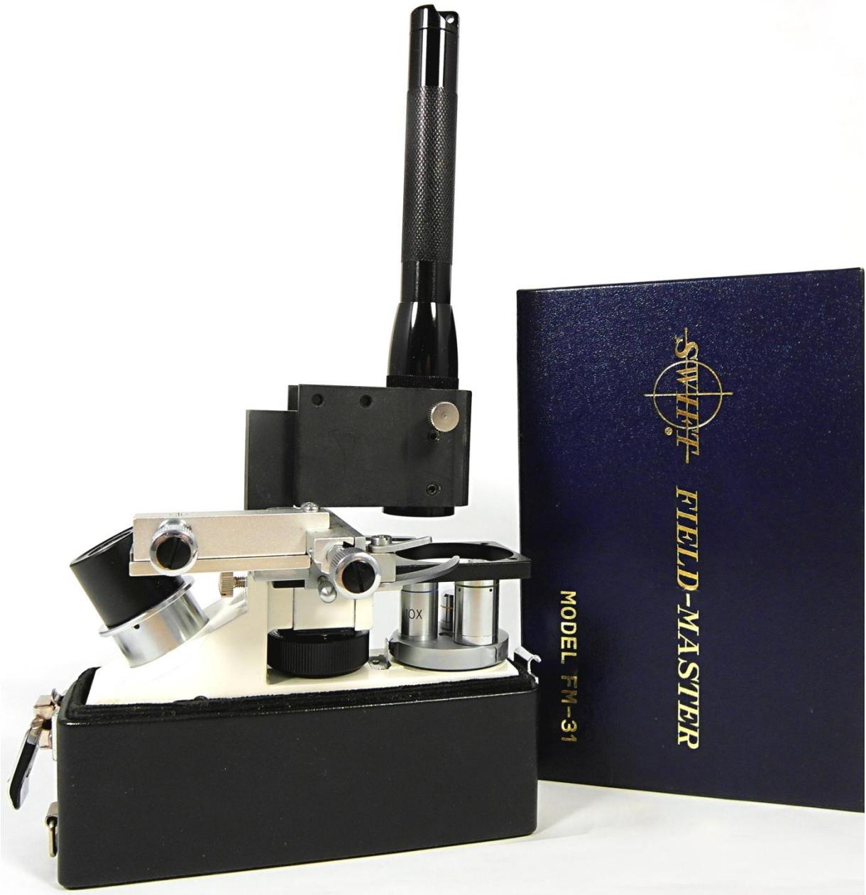
Figure 7. Swift FM-31 with Maglite ® illumination c. 1980s
