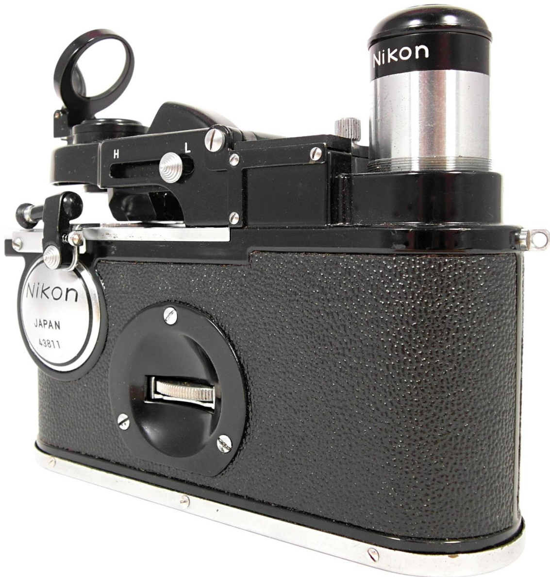
Figure 5. Nikon H folded-optics microscope, c. 1960s
