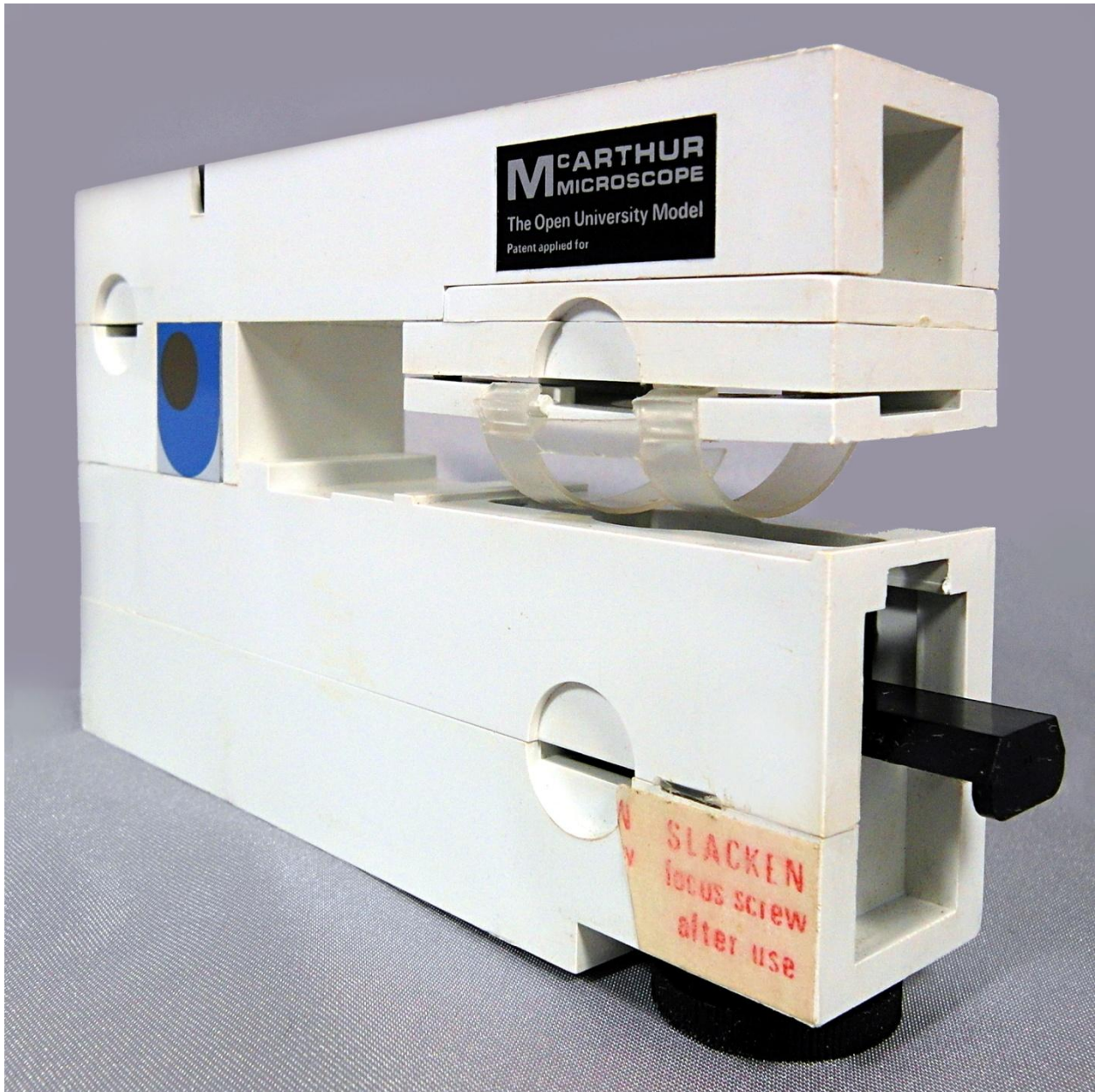
Figure 2. Plastic body McArthur microscope made for the Open University (OU), c. 1970s
