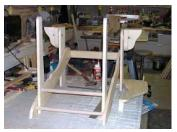
${f 6}$  - Assemble the back supports parts  ${f E}$  with the dowel  ${f F}$ , cut to length. Screw the dowel in place with 2" (5.1cm) screws, being sure the back supports are square to each other. Place the assembled section in front of the rear dowel part  ${f B}$ , being sure that the straight perpendicular front of the assembly, is facing the front of the chair.
