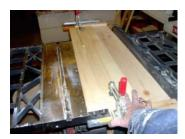
${f 2}$  - A taper jig on the table saw, works best for the back slats and back supports E. A shop built sled is the quickest, easiest and safest taper jig. Use a scrap length of 6" (15.8 cm) wide plywood, longer than back slat  ${f N}$ , and fasten clamps at each end. Line up the pattern line to the edge of the jig, using an adjustable square, and run it through the blade.
