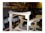
**8** - Assemble the back support pivot parts  $\mathbf{K}$  in the upper holes on the inside of back supports  $\mathbf{E}$ . Be sure that the tops are angled towards the back of the chair. Center the back support part  $\mathbf{L}$  on the pivots, drill pilot holes, **glue** and screw in place with two 2" (5.1cm) screws into each pivot.
