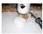
**6** - Using the UHCW plastic, make 8 washers using the 1 5/8" (4 cm) hole saw. The Lee Valley plastic is already 1/4" (6.5mm), but if you buy 3/8" (9.5mm) plastic jig stock at Rockler, rip or plane it to size. Use a cutting blade to trim off the plastic burrs to make the washer smooth.
