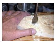
**5** - Using a 7/8" (2.2cm) spade or Forstner bit, drill the 1/4" (6.5mm) deep holes for the dowels in parts **A & E. NOTE:** Be sure to drill the holes on the **INSIDE** of each part. The back supports, parts **E**, are square at the front & angled at the back, so lay them together, then open like a book, and mark the hole locations on the inside.
