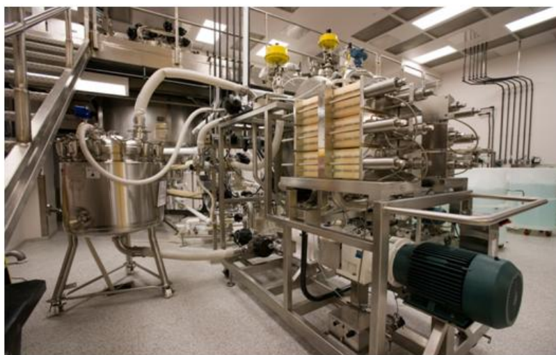
Fig. 26.4: Large scale tangential flow filtration methods ( www.biomanufacturing.com )
