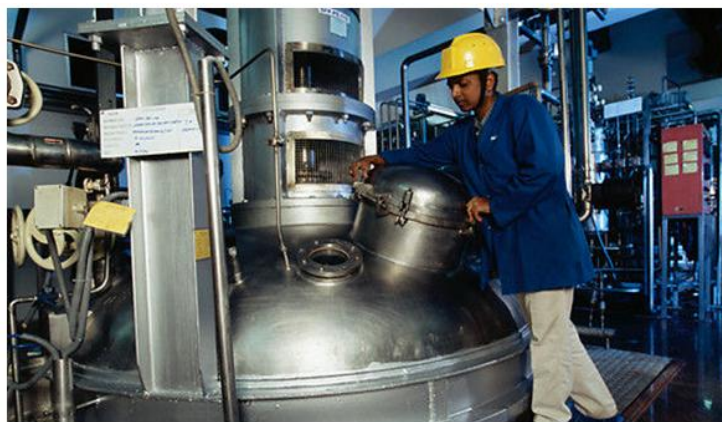
Fig. 22.1: Submerged fermentation unit ( www.biocon.com )
