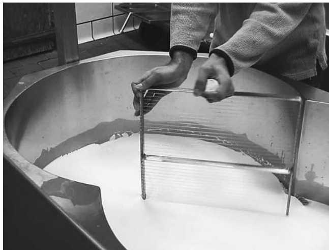
Figure 10.2. Cutting of rennet curd.
