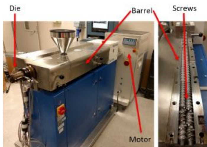
Figure 4. Components of an extruder (CW Brabender 20mm TSE at the WSU Food Extrusion Laboratory).
