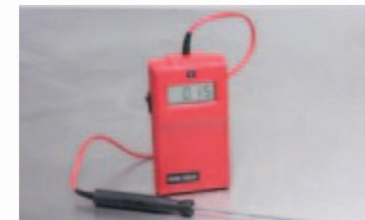
Figure 26 A typical temperature probe
