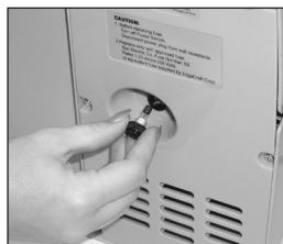
Figure 10. Replacing the fuse located underneath motor housing.
