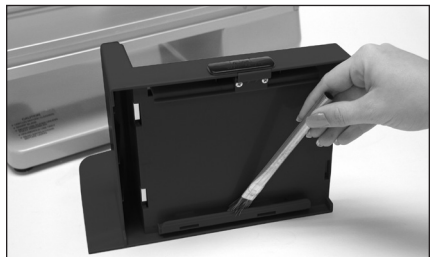
Figure 6. Lubricating food carriage guides.
