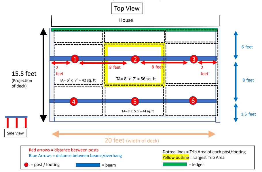
Note this deck has a ledger (green), which means the deck is connected to the house, which will carry part of the load.
