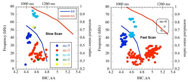
FIG. 4. Frequencies and poloidal mode numbers as a function of the currents in the helical conductor in slow (left) and fast (right) scan discharges. The corresponding times of the discharges are shown above.
