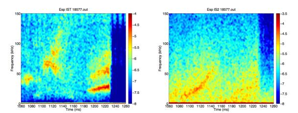
FIG. 5. Spectrograms of the signals of a magnetic probe ( $\rho \approx 1.05$ , left) and the saturation current of a Langmuir probe ( $\rho \approx 0.95$ , right) for the fast scan discharge TJ-II #18577. The discharge is terminated at t  $\approx 1230$  ms due to ECH density cut-off limit.
