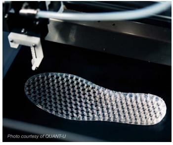
Figure 5. LAM 3D printing of silicone midsole
