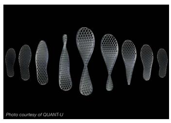
Figure 2. Mass customization potential with 3D printing
