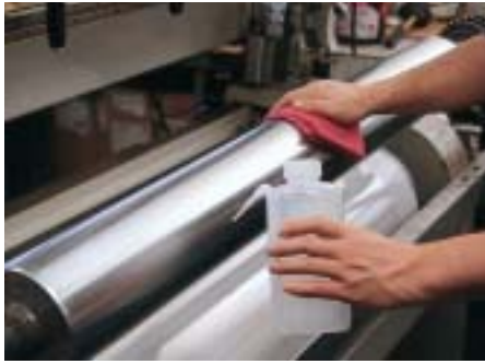
Insure cylinder is clean prior to mounting tape. Allow sufficient time for cleaning solution to dry.
