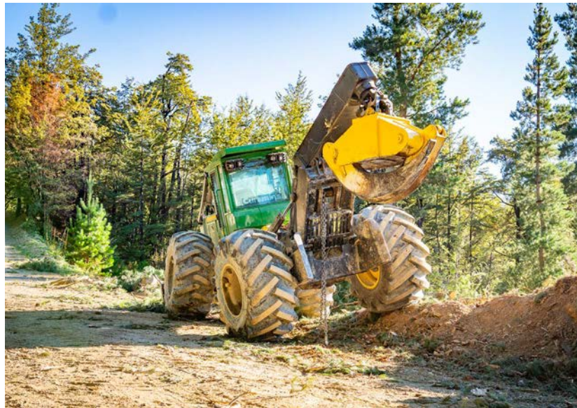
Extraction machine-skidder with winch plus grapple gives flexibility in breaking out individually felled trees with minimal damage to the residual crop.
